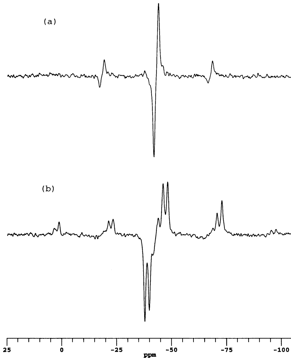
FIG. 2. ^{27}\text{Al} \rightarrow ^{31}\text{P} INEPT spectra of \text{TMP-AlCl}_3 complex in zeolite NaX obtained when ^{27}\text{Al} \Theta = \pi/6 and 2\Theta = \pi/3 pulses ( 1.5 and 3.0 \mu\text{s} ) were applied (a) asynchronously and (b) synchronously with the rotor period. Evolution times ( \tau ) of 0.75 and 0.833 ms were used, respectively. Spinning speed = 3.6 kHz; ^{27}\text{Al} RF strength = 55 kHz. Spectra have been plotted on the same scale.
